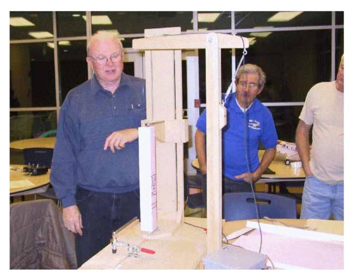
At the January Meeting, Jim Halbert demonstrates the foam cutting machine that he developed. It cuts both cylinders and cones, and they can be solid or hollow. He also has a large foam cutter at home that he uses to cut foam wing cores. He brought samples of the wing cores and some templates used to cut different airfoils. Shown are Jim Halbert on the left, Jack McEvoy center and Gene Fuson on the right.
