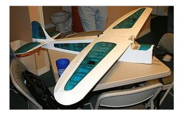
Greg Moody brought his Aviator Pro 60 ARF to the March meeting. Looking a little like a SIG Rascal, the plane has a 68 inch wingspan and Greg plans to put a four stroke engine in it. The plane is intended to fly like a trainer.
