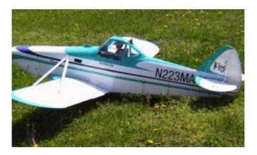
Above are photos of Sid Beckham's Hanger 9 Piper Pawnee ARF on its maiden flight and just after landing. This 80 inch wing span model is a faithful and great looking representation of the actual plane. Sid has a .46 2-stroke in it which is at the low end of the power recommendation, however, it flew quite well. Actually fairly slow but very steady.
