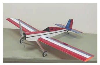
Above is Jim Halbert's 3 Star E based on the 4 Star 40. Reduced to 80 % and customized. It is powered with an AXI 2822/12 motor and someday a 2450 mAH Li-Po battery. Nice looking airplane!
