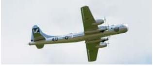
The Pilot's Choice award went to this B-29. It has about a six foot span and was covered in aluminum foil and had lots of panel lines and details. Flew well in the wind
