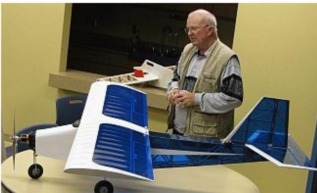
Above is Jim Halbert's electric Super Cadet. The 80 inch wing is ARF and the rest is sort'a plan built. With a Scorpion 4020-16 outrunner motor and nine A123 cells (about 35 volts) it should put out about 700 watts (1 Hp) at 20 amps. It should fly well and stay up around 10 minutes at a little over half throttle.
