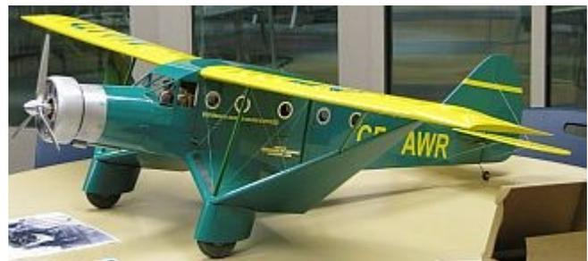
Above is Don Johnson's latest and maybe last, Bellanca Aircruiser. Scratch built from his own plans it has a span of 65 inches and has a flying weight of 48 ounces (3 pounds). It has a Scorpion 3008-26 outrunner motor and a 3 cell 3700 mAH Li-Po battery. At 37 amps it develops over 370 watts, or over 120 watts per pound. The large letters are hand cut and the small ones are custom made decals. Now for a nice calm day at the field!
