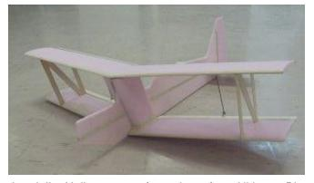
Lend Jim Halbert a set of templates for a Ultimate Bipe designed for 1/4" fan fold foam and what happens. It turns out to have wings with airfoil and dihedral. The wing strut in front of the cockpit looks to be a little draggy Jim! How about a fly off between a flat wing and the airfoil wing?
