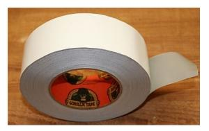
The bottom of the fuselage and floats need some protection since taking off the ground would soon chew up the foam. The Scotch TOUGH tape is thick, transparent and tough and has a white web reinforcement in it. It also stuck very well to the painted bottom surfaces. Another possibility is the GORILLA TAPE. It is a multilayer duck tape and comes in white and black. Didn't use this on the Polaris but should work well.
