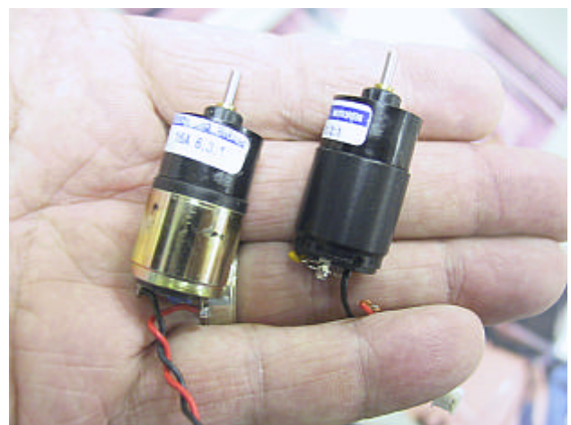
Above are a couple of motors that are used to power the Daimler-Chrysler flying cars that John Woods flies. It only takes three of these tiny motors to fly the 80% scale cars.
