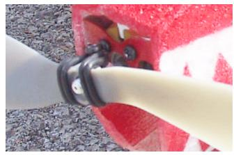
Above note the prop mounting. The prop adapter is cut off and the prop held to the back of the adapter with two 3/32 inch o-rings overlong set screws. This allows the prop to deflect about 30 degrees in a hard landing.
