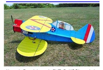
Above is Don Johnson's PVT. B. KOOL made by somewhat following a Model Aviation mag plan. The wings are 3 mm Depron and everything else is 6 mm Depron. It has a 32 inch wingspan and weighs about 19 ounces. Except for the star decals, the model is hand painted with cheap acrylic paint from Wal-Mart and panel lined with a black gel pen. The motor is an AXi 2212/34 with a Phoenix 10 speed control and 1050 mAH Li-Poly 3-cell battery. Photo by Annette McEvoy.
