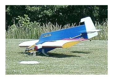
Above is Erv Rohde'S Pro Twister touching down very close to the target. Note that the landing gear is bent up far enough so the fuselage is actually touching the ground—and the landing gear did not break, Picture by Fritz Corbin.
