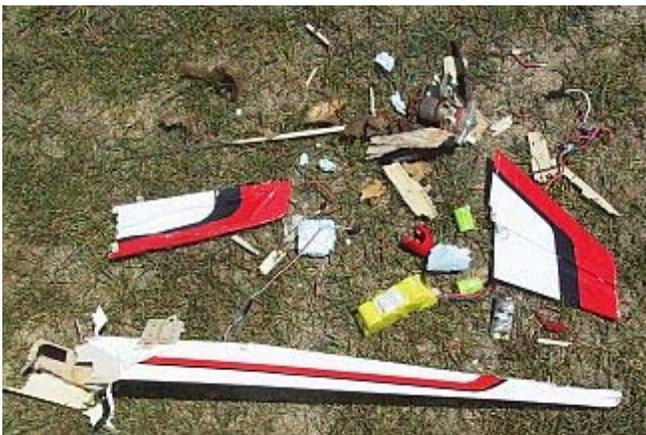
box, receiver and speed control had been destroyed—over a \$350 loss. Salvageable was the folding prop, two micro servos (had to replace one set of gears) and eight out of the nine NiMH battery cells. Most of the cells were dented but seem serviceable.
