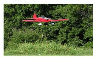
Below is Don Johnson's newest project. Shown in bare bones, the Stinson Reliant is an old 25 cent Comet kit with a 25 inch span. It will be 3 channel R/C and use the Park Zone Brick, a 5 gram outrunner and 2 cell 300 mAH Li-Po. Hopefully it will weigh in at 2.5 ounces or less.
