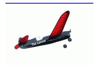
The Lancer flies in the south Texas skies at BEST. Don Johnson's early 40's designed gas free flight, which he converted to an electric RC, heads up at New Waverly Texas. It's not very maneuverable due to the small rudder, but with a six foot wing span and light weight it does have a nice floating glide. A great plane for older flyers.
